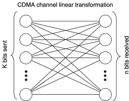
Fig. 1. Factor graph describing the linear channel
