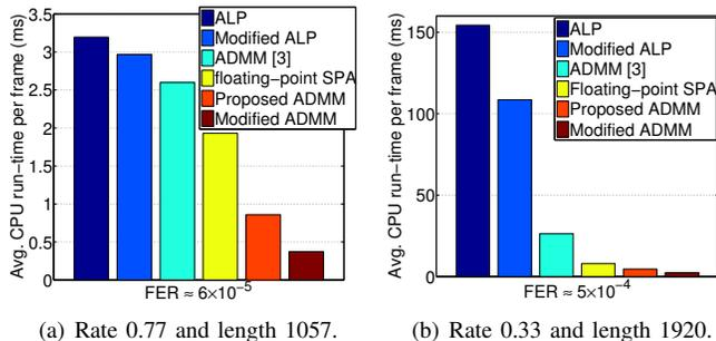
Fig. 2. Average simulation time for decoding one codeword.
