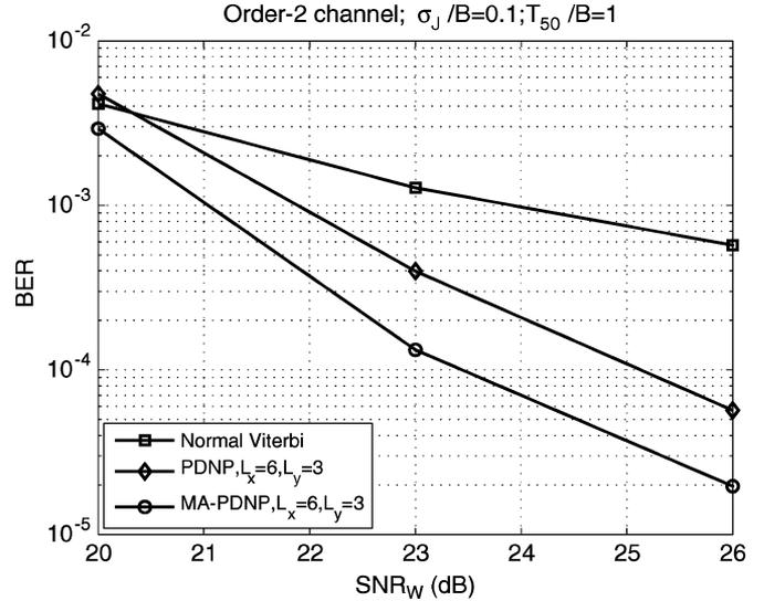
Fig. 2. Comparison between Viterbi, PDNP, and MA-PDNP detectors.
