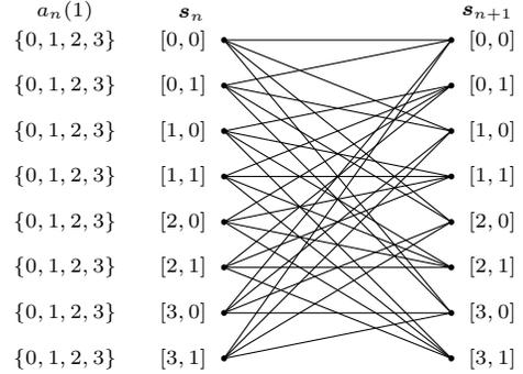
Fig. 6. Subset trellis with configuration [4,2] on memory-2 channel.
