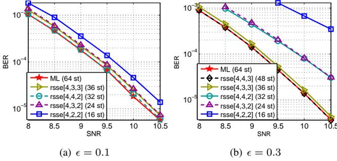
Fig. 7. Performance comparison between RSSE and ML detector on EPR4 channel at different ITI levels. The legend shows the RSSE subset trellis configuration and the corresponding number of trellis states.
