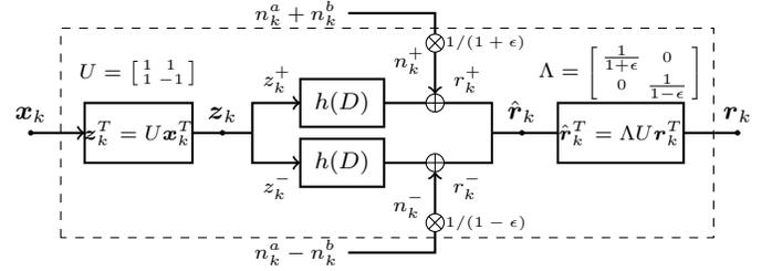
Fig. 2. A schematic of the WSSJD model. Coordinate transformations are applied in the input space ( $\mathbf{z}_k^T = U\mathbf{x}_k^T$ ) and the output space ( $\hat{\mathbf{r}}_k^T = \Lambda U\mathbf{r}_k^T$ ). They decompose the original 2H2T system into the sum channel (upper branch) and the subtract channel (lower branch).
