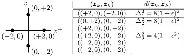
Fig. 3. The input constellation (left) and the ESPDs (right).
