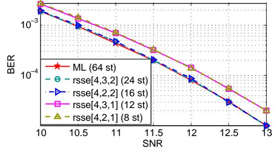
Fig. 8. Performance comparison between RSSE and ML detector on minimum phase channel  $h(D) = 1 + 1.6D + 1.1D^2 + 0.4D^3$ , at  $\epsilon = 0.1$ .
