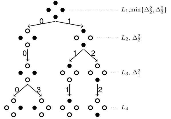
Fig. 5. The modified set partition tree. This tree contains 4 levels,  $\{L_1, L_2, L_3, L_4\}$ , each of which is a set partition of the WSSJD input constellation. The minimum ESPD on each level is specified on the right side. The number associated with each branch is the index of the subset in the corresponding set partition.
