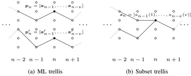
Fig. 1. Comparison between the decoding paths on (a) ML trellis and (b) subset trellis. If at time  $n$  two paths ending at ML states  $\mathbf{p}_n$  and  $\mathbf{p}'_n$  satisfy  $\mathbf{x}_{n-k} \in a_{n-k}(k)$  and  $\mathbf{x}'_{n-k} \in a_{n-k}(k)$  for all  $k = 1, \dots, \nu$ , then they will merge early at subset state  $\mathbf{s}_n$  in the subset trellis.
