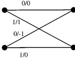
Fig. 2. Trellis section for the dicode channel.
