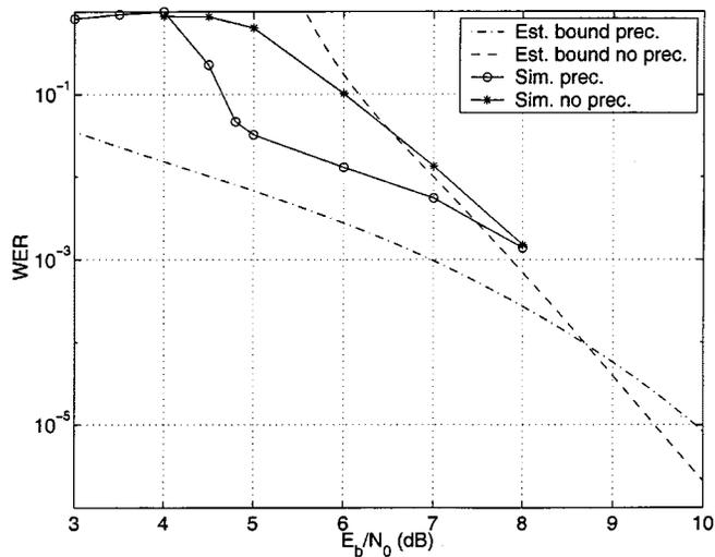
Fig. 4. WER union bound estimates and simulation results for outer convolutional code.
