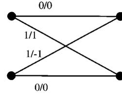
Fig. 3. Trellis section for the precoded dicode channel.
