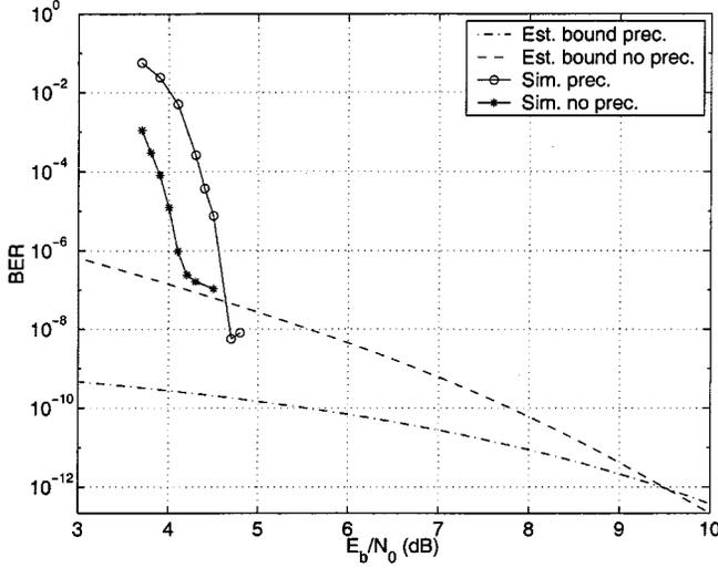
Fig. 7. BER bound estimates versus simulation results for precoded and nonprecoded turbo system.
