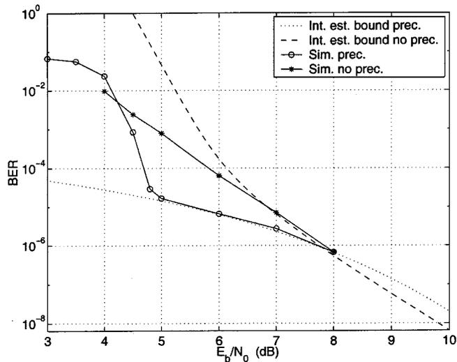
Fig. 6. Truncated bound estimates for interleaver used versus simulation result for outer convolutional code.
