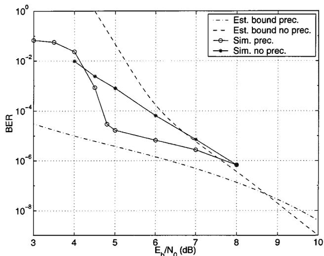
Fig. 5. BER union bound estimates and simulation results for outer convolutional code.
