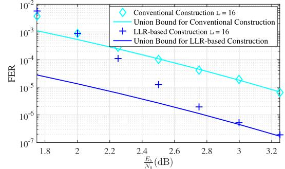
Fig. 6. Union bound approximation (5) and FER for CRC-aided SCL decoding.
