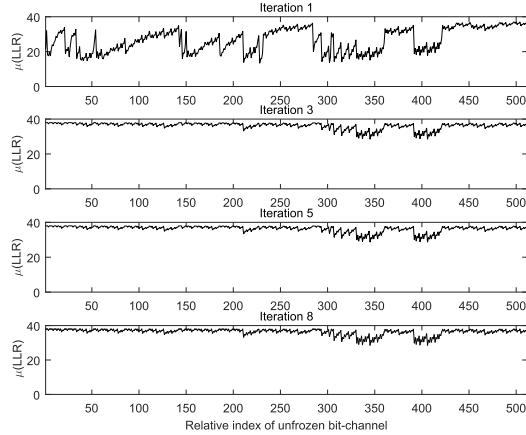
Fig. 2. Mean LLR values ( $\mu(\text{LLR})$ ) under BP SCAN decoding of unfrozen bits of polar code in Fig. 1 after LLR-based bit-swapping of 12 bit-channels, on AWGN channel,  $\frac{E_b}{N_0} = 2.25 \text{ dB}$ .
