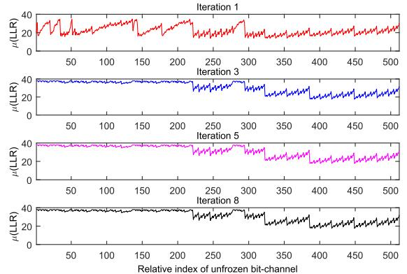
Fig. 1. Mean LLR values ( $\mu(LLR)$ ) under BP SCAN decoding of unfrozen bits of polar code with  $N = 1024$ ,  $R = \frac{1}{2}$ , on AWGN channel, with  $\frac{E_b}{N_0} = 2.25$  dB. Code optimized at  $\frac{E_b}{N_0} = 2.25$  dB according to [13].
