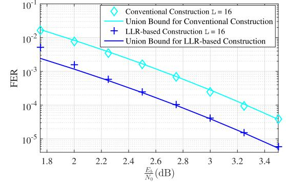
Fig. 5. Union bound approximation (5) and FER for SCL decoding.
