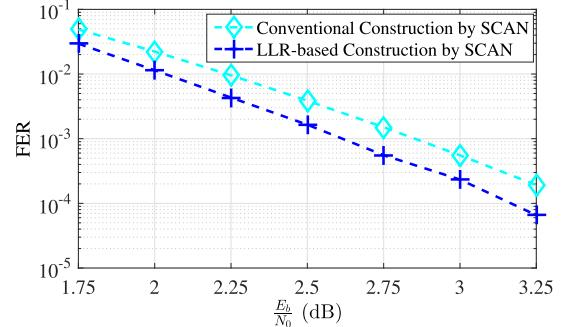
Fig. 4. FER of conventional and LLR-based polar codes under BP SCAN decoding on the AWGN channel.
