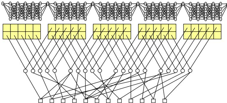
**Figure 9.** Decoding graph for joint IMS detection and message-passing LDPC decoding.
