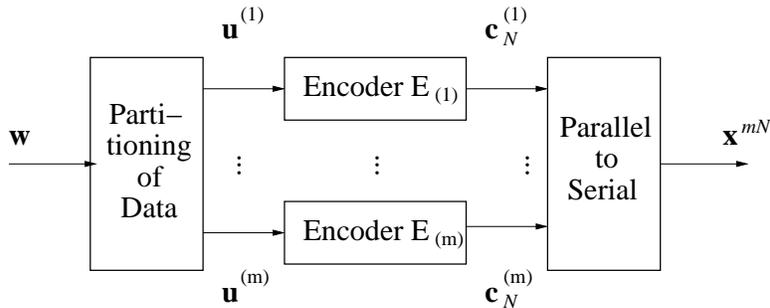
Figure 2. Multilevel encoder architecture.
