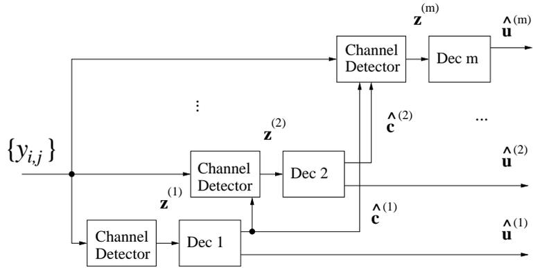
Figure 3. Multistage decoder architecture.
