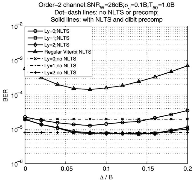
Fig. 4. MA-PDNP detector with dibit precompensation.
